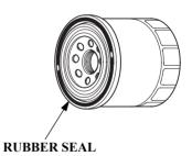
4. Clean the oil filter mounting base, and coat the rubber seal of the new oil filter with clean engine oil.
