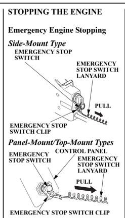
To stop the engine in an emergency, pull the emergency stop switch clip out of the emergency stop switch by pulling the emergency stop switch lanyard.
