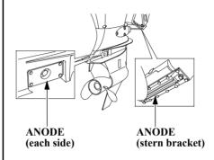
The anodes are made of a sacrificial material that helps to protect the outboard motor from corrosion.
