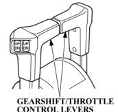
The gearshift/throttle control lever(s) controls engine speed and selects F (forward), N (neutral), or R (reverse) gears.
