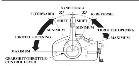
Moving the control lever 32° from N (neutral) selects the gear, and further movement increases engine speed.
