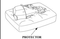
If it is necessary to store the outboard motor horizontally as shown, drain the vapor separator (p. 88), and drain the engine oil (p. 67), before removing the outboard motor from the boat
