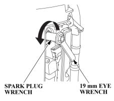
9. Remove the spark plugs with a spark plug wrench and 19 mm eye wrench.
