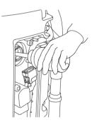
5. Pour a teaspoon (p. 89) of engine oil into each spark plug hole to lubricate the inside of the cylinders. Reinstall the spark plugs.
