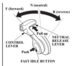
The fast idle button allows you to increase the idle speed without engaging the drive gears. Move the control lever forward or reverse after pushing in the fast idle button to increase the idle speed.
