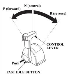
The fast idle button allows you to increase the idle speed without engaging the drive gears. Move the control lever forward or reverse after
