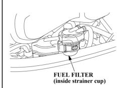
2. Looking through the translucent strainer cup, check the fuel filter for water accumulation or sediment.
