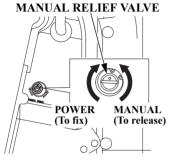
The outboard motor can be tilted manually after opening the manual relief valve. This feature enables the outboard motor to be tilted up or down when no battery is connected.
