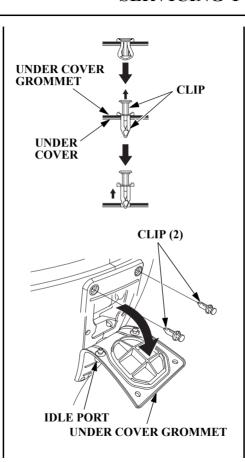
3. Remove the two clips from the upper part of the under cover grommet.
