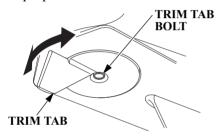
Adjust the trim tab with the engine stopped. Loosen the bolt above the trim tab, turn the trim tab, and then tighten the bolt securely.
