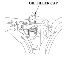
4. If the oil level is low, remove the oil filler cap, and add oil to reach the upper limit mark shown on the dipstick. Use the oil recommended on p. 70.
