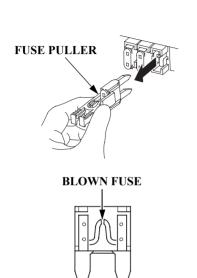
4. Use the fuse puller from the fuse holder to remove the fuses. If a fuse is blown, install a replacement fuse of the same specified rating.
