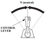
1. Move the control lever(s) to the N (neutral) position.
