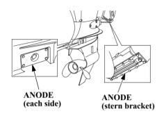
The anodes are located on each side of the gear case and on the stern bracket. They are made of a sacrificial material that helps to protect the outboard motor from corrosion
