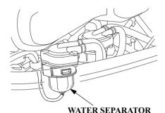
When the water separator buzzer sounds (a rapid, repeating signal):
