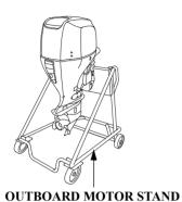
If the outboard motor will be removed from the boat for storage, we recommend storing it vertically by mounting it on a commercially available stand.
