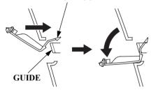
3. Set the drain bolt cover under the guide.
