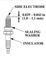
11. Measure the spark plug electrode gap with a wire-type feeler gauge. Correct the gap, if necessary, by carefully bending the side electrode.
