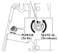
The outboard motor can be tilted manually after opening the manual relief valve. This allows the outboard motor to be tilted up or down when no battery is connected.
