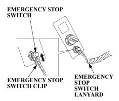
1. Put the emergency stop switch clip in the emergency stop switch, and attach the emergency stop switch lanyard securely to the operator or to the operator's PFD (Personal Flotation Device).
