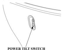
The power tilt switch is located on the engine pan. It is a rocker switch with UP and DN (down) positions for changing the angle of the outboard motor.
