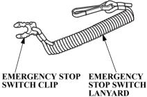
The emergency stop switch clip must be inserted in the emergency stop switch in order for the engine to start and run. The emergency stop switch lanyard must be attached securely to the operator or to the operator's PFD (Personal Flotation Device).
