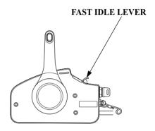
Use the fast idle lever to accelerate engine warm-up after starting the engine. Do not use the fast idle lever when starting the engine.
