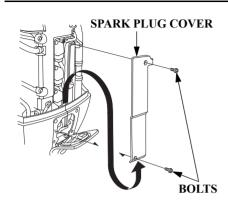
5. Remove the two bolts with the 6 mm hex. wrench, and remove the spark plug cover.
