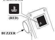
If the engine overheats, the overheat indicator will come on, and the engine will stop in 20 seconds after the engine protection system limits engine speed. If you are at cruising speed, engine speed will decrease automatically.
