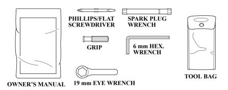
The tool kit can be used for simple maintenance procedures and emergency repairs. Keep these items on the boat so that they will always be available if you need them.
