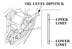
3. Insert the dipstick all the way in, then remove it and check the oil level shown on the dipstick.
