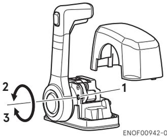
1. Throttle friction adjustment screw
