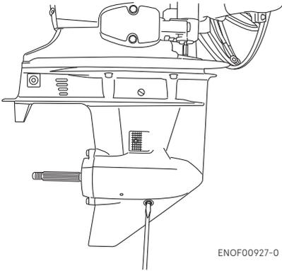
3. Insert the oil tube nozzle into the lower oil plug hole, and fill with gear oil by squeezing the oil tube until oil flows out of the upper plug hole and bubbles is disappeared to remove the air.
