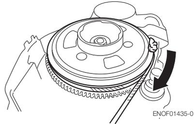
5. Tie a loop in the another end of the emergency starter rope and attach socket wrench that is included in the tool kit.
