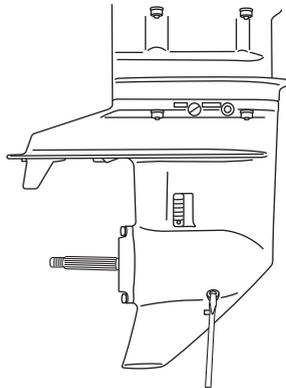
3. Insert the oil tube nozzle into the lower oil plug hole, and fill with gear oil by squeezing the oil tube until oil flows out of the upper plug hole and bubbles is disappeared to remove the air.
