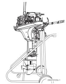
Keep the outboard motor in a vertical position when mounting.
