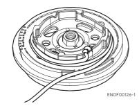
6. Tie a loop in the another end of the emergency starter rope and attach socket wrench, Both the loop and the wrench are provided in outboard motor box.
