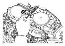
4. Remove the bolts (3pcs) and remove the recoil starter.
