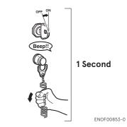
2. Within 5-10 seconds, Pull the red knob on the safety switch out and release.
