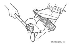
5. Install a new split pin into the nut hole and bend it.
