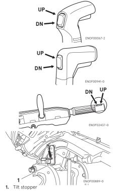
The outboard motor can also be tilted up and down using the switch provided on the bottom cowl.
