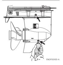
4. Install the upper oil plug, and then remove oil tube nozzle and install the lower oil plug.
